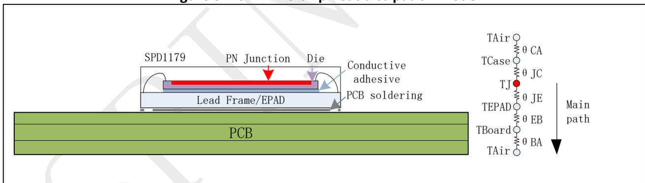
The junction temperature measurement and overtemperature protection of the chip can be carried out by using the integrated PN junction temperature sensor in the chip. The junction temperature of the chip can also be calculated by ① calculating the power consumption of the chip and ② measuring or calculating the ring thermal resistance of the system, and then the junction temperature of the chip can be calculated by using **Formula 3.1**.
