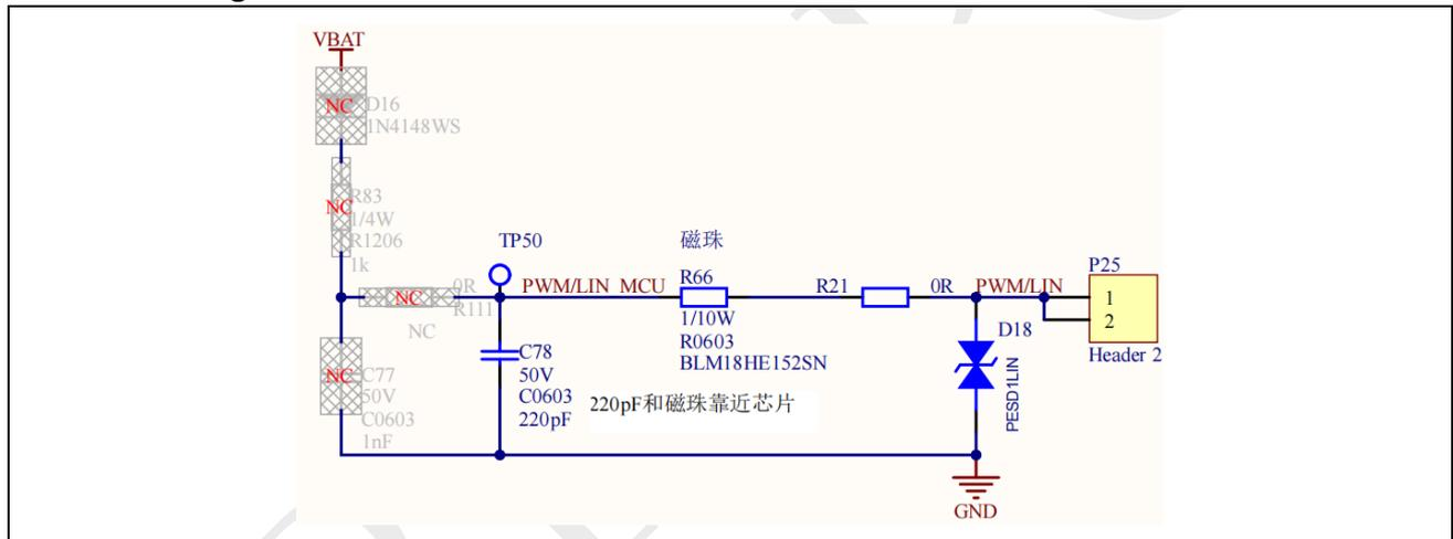
As shown in Figure 1-12, it is the recommended circuit for SPD1179 in master mode of the LIN interface. In Master mode, it is necessary to select appropriate pull-up resistor and ground capacitor values to ensure that the waveform slope in LIN conformance test meets the specification requirements. Generally, 1K pull-up resistor and 1nF ground capacitor are used, as shown in R83 and C77 in Figure 1-12. In this case, the R111 resistor needs to be welded and the capacitor C78 needs to be removed.
