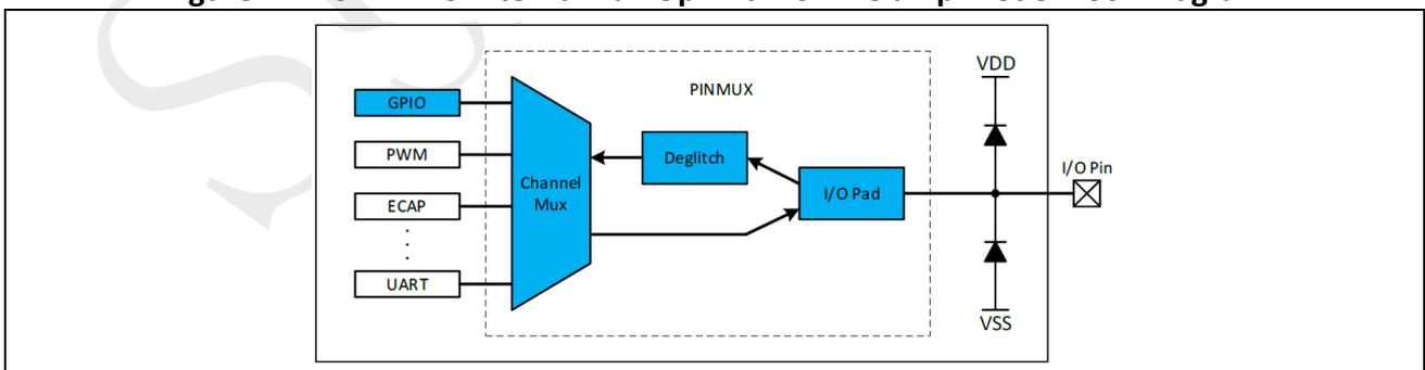
When the IO port input voltage is higher than the internal clamp supply voltage, then the diode clamp action will occur, there will be a feed current from the IO port into the 5V or 3.3V supply. This is often encountered in automotive key signal detection, where the high-level key signal is the battery voltage (9-16V) and the low-level is 0V.
