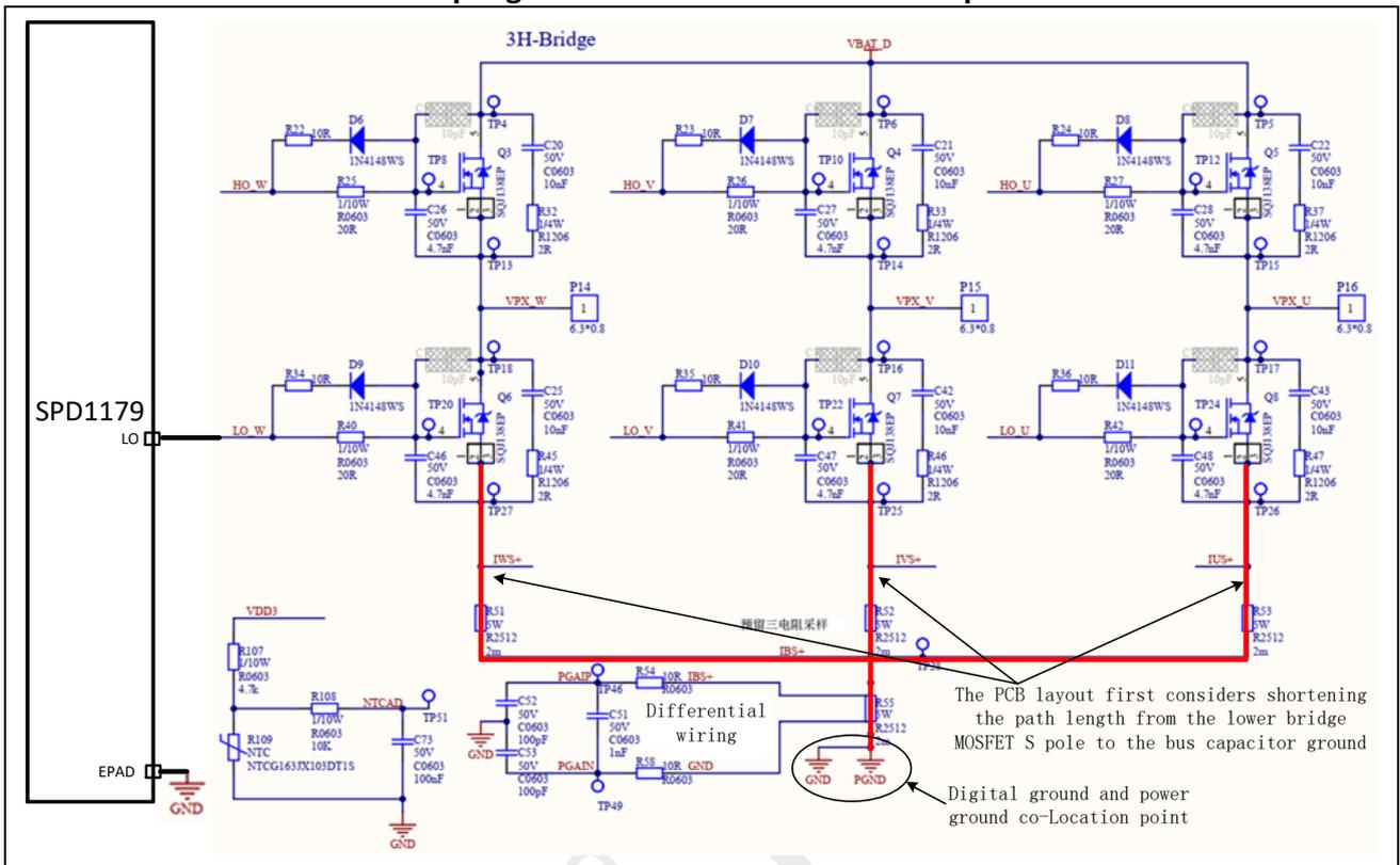
**Figure 4-2 Shorten the length of the low-side bridge S pole to the sampling resistor to the bus capacitor track PCB example**
