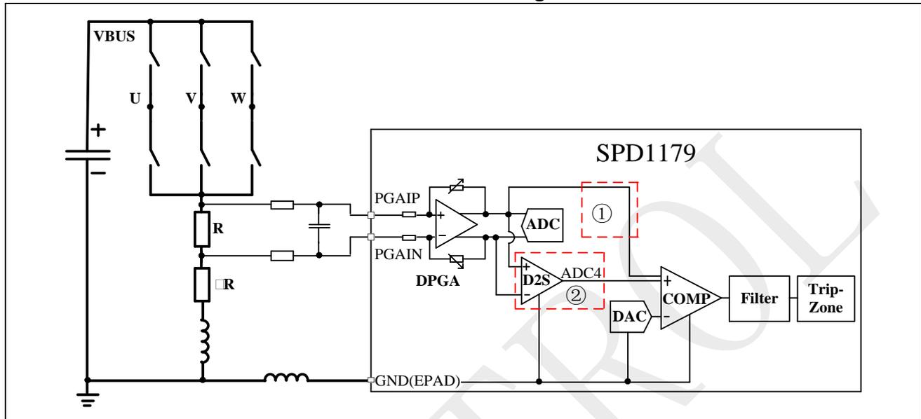
There are two ways to configure the internal comparator overcurrent protection.
